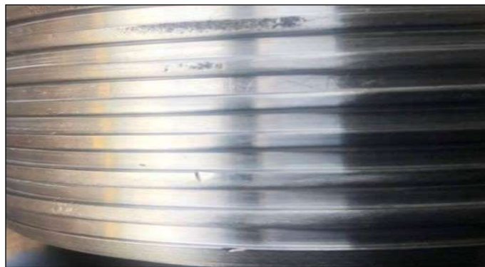
Photo. 4 Dings on crest of the threads/Golpes en crestas
