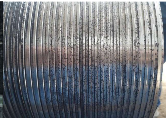
Photo. 16 Major oxidation: Rejected
