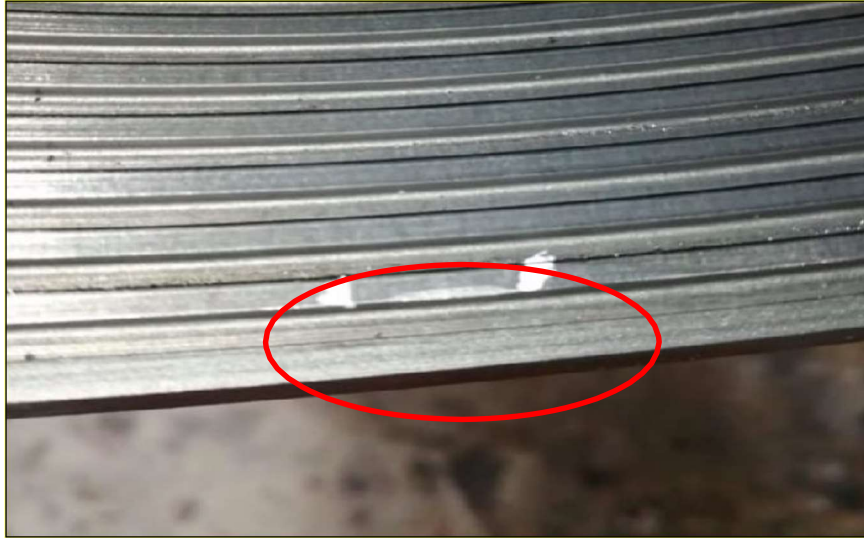
Photo.14 Dings on the crest of the thread without affecting the load flank: Can be repaired
