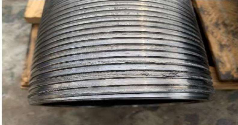
Photo. 5 Galling in a pin connection after a make-up
