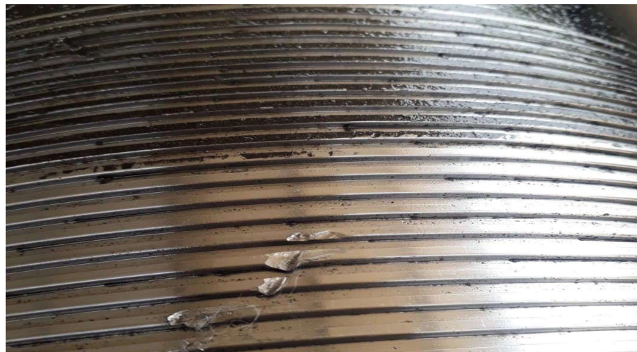
Photo.13 Longitudinal major cuts on a pin connection: Rejected
